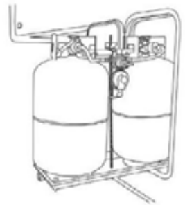
Two Propane Cylinders
