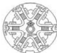
7-way trailer plug car end, rear view
