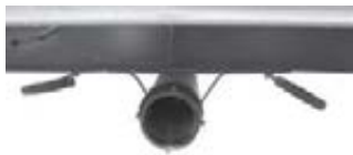
Black/Grey Tank Drain and Valves
