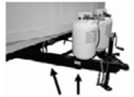
Electrical wiring & safety break-a-way switch Detachables Hitch
