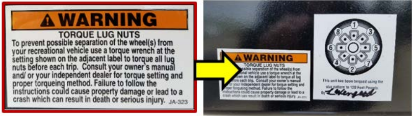
Lug nut torque pattern and warning label
